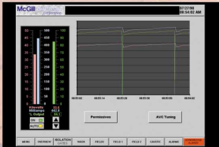
The PC-SAM control system has extensive reporting and trending capabilities, including on-screen operation and maintenance manuals.
