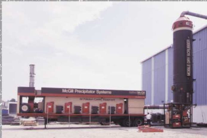
A McGill AirClean mobile EP and spray-dry scrubber can be used to test emissions and analyze your control needs.
