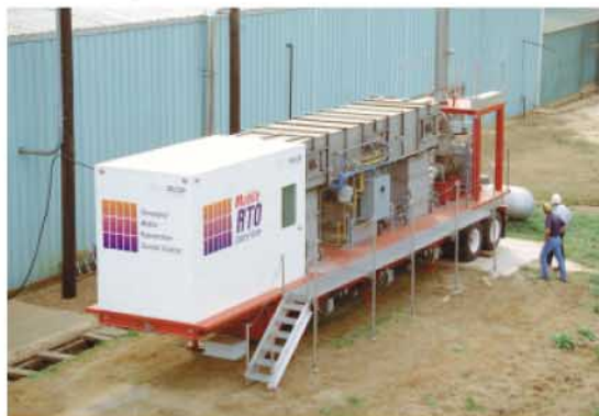
6. The mobile RTO is ready to begin testing your process emissions.
