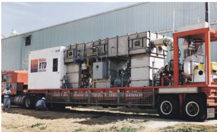
1. Very little room is needed for the mobile RTO trailer. It is equipped with self-leveling hydraulic jacks so that it can be set up on a variety of surfaces.
