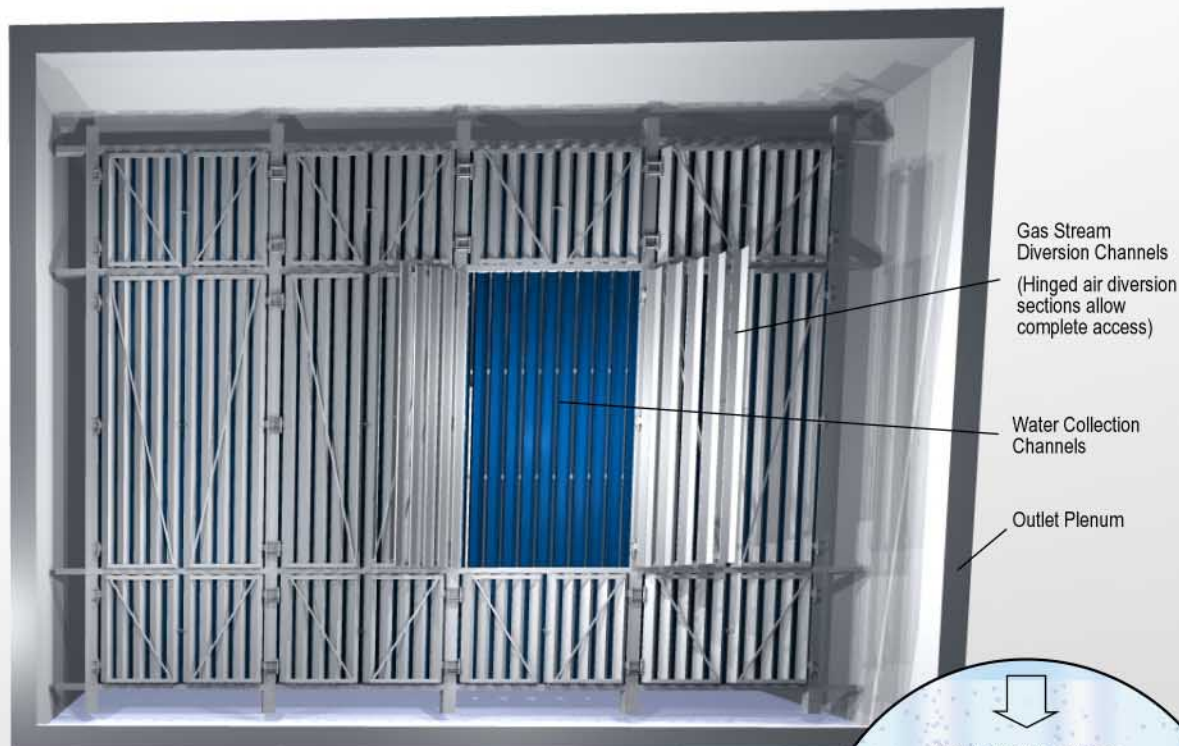
Drawing of a McGill AirClean mist elimination device installed in the outlet plenum of a McGill wet EP. Note the hinged sections that provide access to all the surfaces of the mist eliminator.
