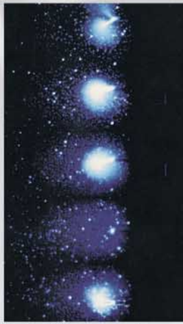
A view of the same needles under normal applied DC voltage. Corona current flows from the needle tips through the gas stream to a resistive layer on the grounded collection plate.
