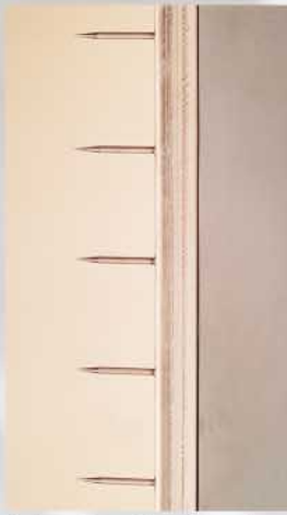
A view of a section of needles mounted on the edge of a high voltage collection plate
