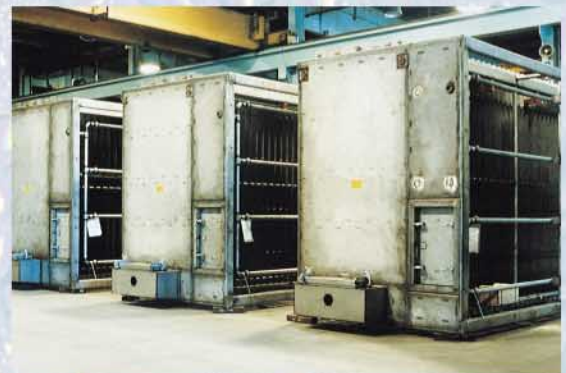
McGill AirClean has the knowledge and experience to properly select the correct materials of construction to meet the particular demands of an application, greatly extending the operation life of the wet EP. Modules shown in McGill AirClean's steel fabricating plant.
