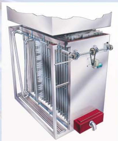
Artist's rendering of a McGill AirClean wet EP module equipped with an optional traveling spray header which may be incorporated when extremely sticky materials must be washed from the collection plates.
